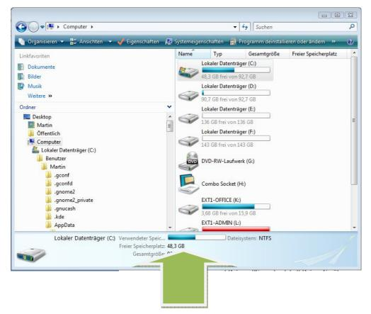
After you have connected to your GPS to the computer, the device should be available here. From here, you can access the devices memory and finally the "Root Directory" and all other files and folders. -Use the "Explorer" on your computer to view and access the memory content of your device. -Use "Notepad" or any other "text editor" to create or modify the "calibration text file(s)".
